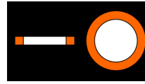
Fig. 3. Profile of a perfectly round vessel (white) in 2D (left) and 3D (right), where the orange visualizes the area when 1/6 higher diameter than the real vessel is segmented.
