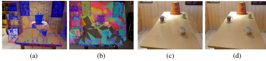
Fig. 3: (a) Segmented overlapping region of a reference image with homogeneous (blue) and inhomogeneous triangles (red); (b) Visualization of a multidimensional per-pixel weight map for an overlapping homogeneous region of a target image. Each homography is represented by a unique color. The pixel color in the overlapping homogeneous region is a combination of colors according to the weighted homographies; (c) Stitching result of an overlapping region. The homogeneous region was transformed and blended. The inhomogeneous region was unprocessed; (d) The same stitching result with color mapping applied to the inhomogeneous region.
