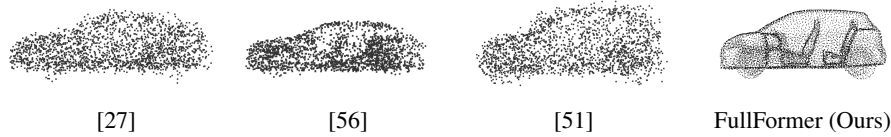
Fig. 6: Generation Comparison: From left to right (Diffusion [27], Point Flow [56], Graph-CNN GAN [51], FullFormer (Ours)). Our model (with 16^3 latent space resolution) shows high-quality internal structure generation results compared to other mentioned models. It is apparent that other comparative models do not achieve discernable internal structures in generation results. All point clouds in this figure are sampled to 2048 points.
